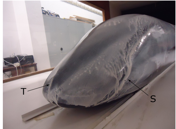
Figure 24: Regions where there appears to be convergence of surface shear stress lines.
