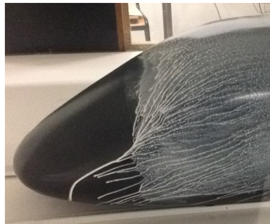
Figure 17: Appearing of the separation region before in an initial phase.
