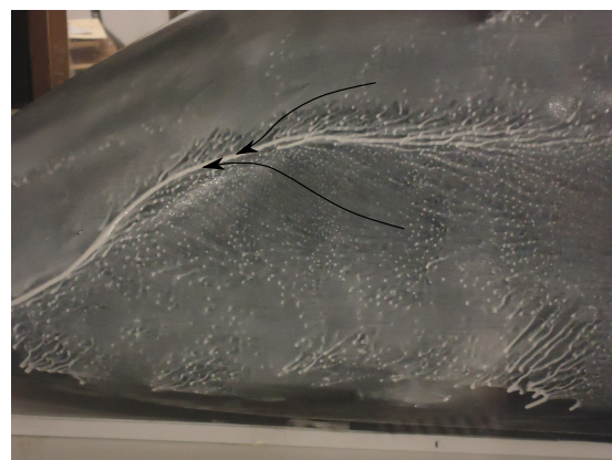
Figure 21: Separation zone in the rear of the model with indication of the local direction of surface current lines.
