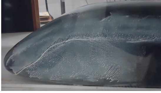
Figure 22: Extension of separation in the rear region.
